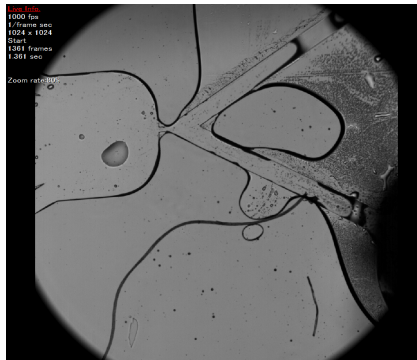
Figure 17: Failed bonding, beads end up outside of the channels.
