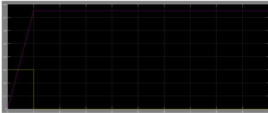
Figure 19: Voltage step response of the cart yellow = input, pink = output
